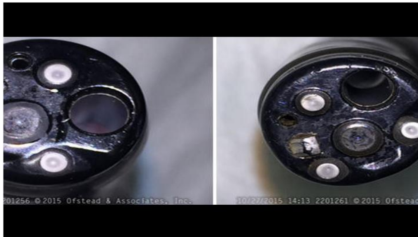
Damaged ends of colonoscopes show scratched, cloudy lenses and, right, dents and brown debris around channel outlets. (Courtesy of Ofstead & Associates Inc., American Journal of Infection Control)
